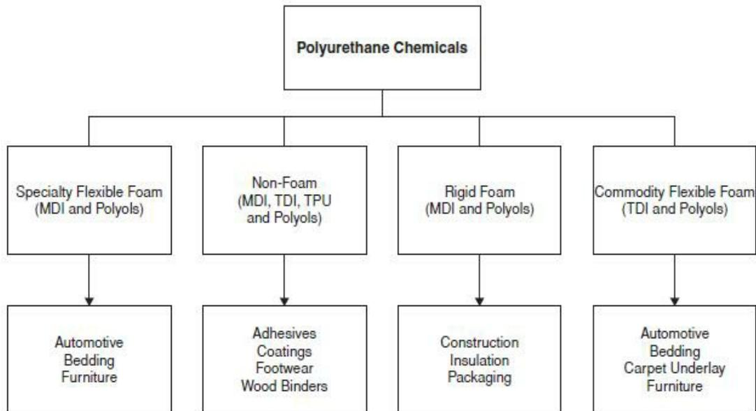
Polyurethane chemicals are sold to customers who combine the chemicals to produce polyurethane products. Depending on their needs, customers will use either component polyurethane chemicals produced for mass sales or polyurethane systems tailored for their specific requirements. By varying the blend, additives and specifications of the polyurethane chemicals, manufacturers are able to develop and produce a breadth and variety of polyurethane products.
